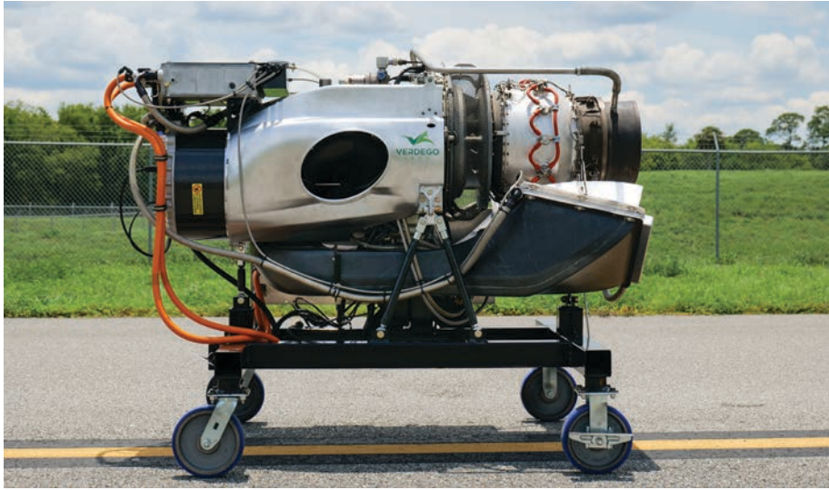
■ VH-4T-RD 400kW (550 hp) turbine hybrid-electric powerplant
