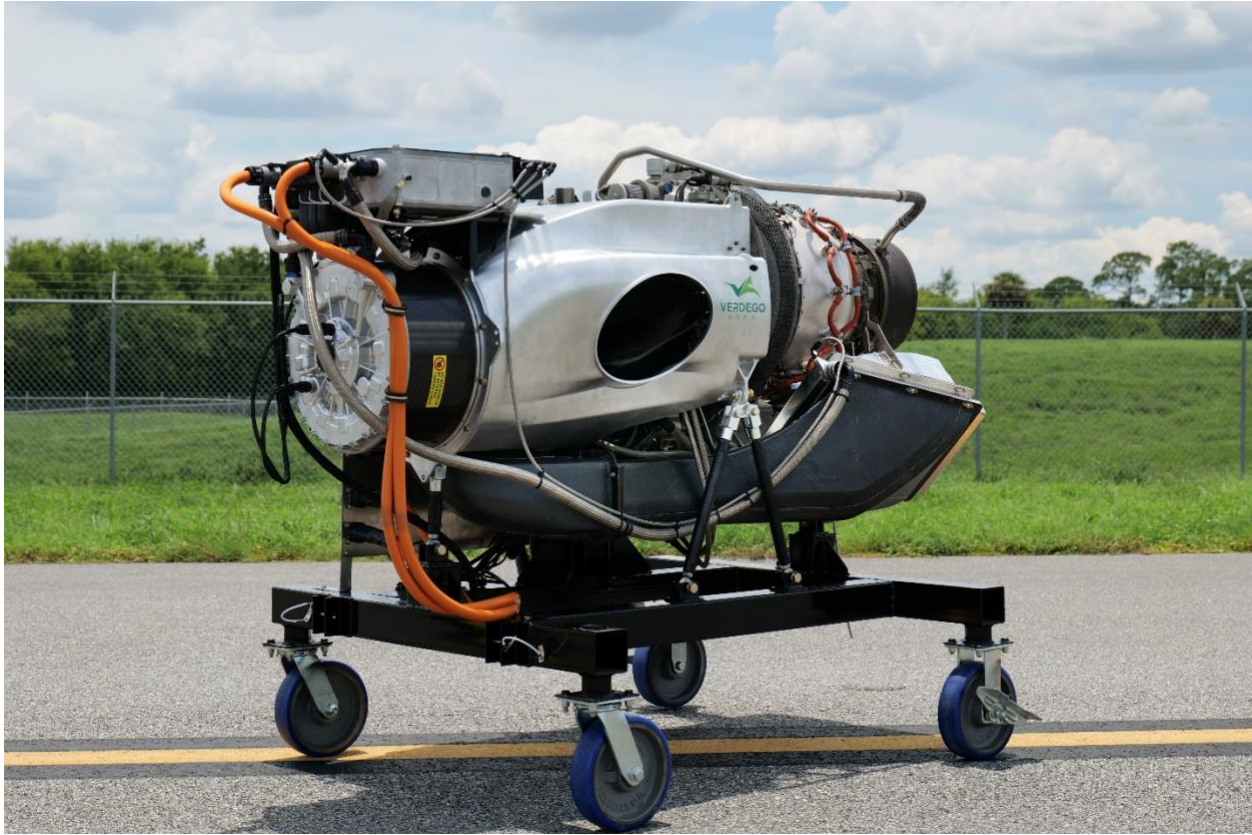
VerdeGo Aero VH-4T-RD 400-kW turbine-hybrid powerplant
